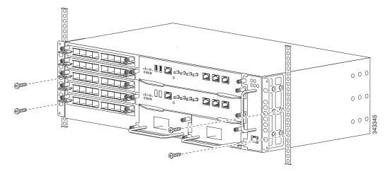
Figure 3-5 Installing the Chassis in a 300 mm ETSI Cabinet
